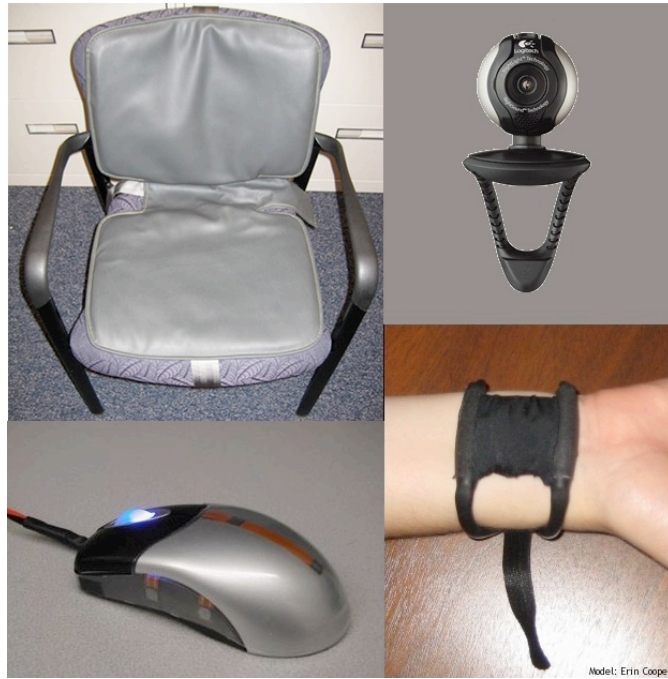
Figure 3. Sensors used in the classroom (clockwise): Facial Expression Sensor; Conductance Bracelet, Pressure Mouse and Posture Analysis Seat.
